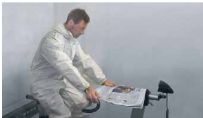
Measurement taken via 10 sensors on the chest and 14 on the back.
